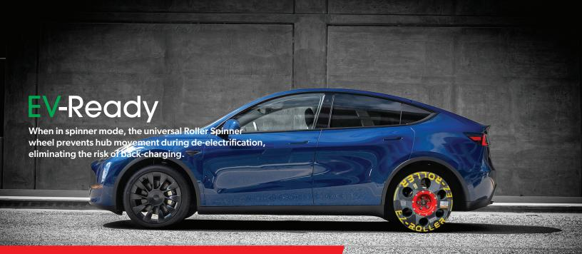
**EZ Roller-Spinner Universal** Wheel offers a unique mobility solution for standard and electric vehicles with frozen brakes or power loss. Easy to use, it bolts onto the vehicle's hub in minutes, enabling the disabled car to be pushed or pulled into a shop or onto a tow truck.
